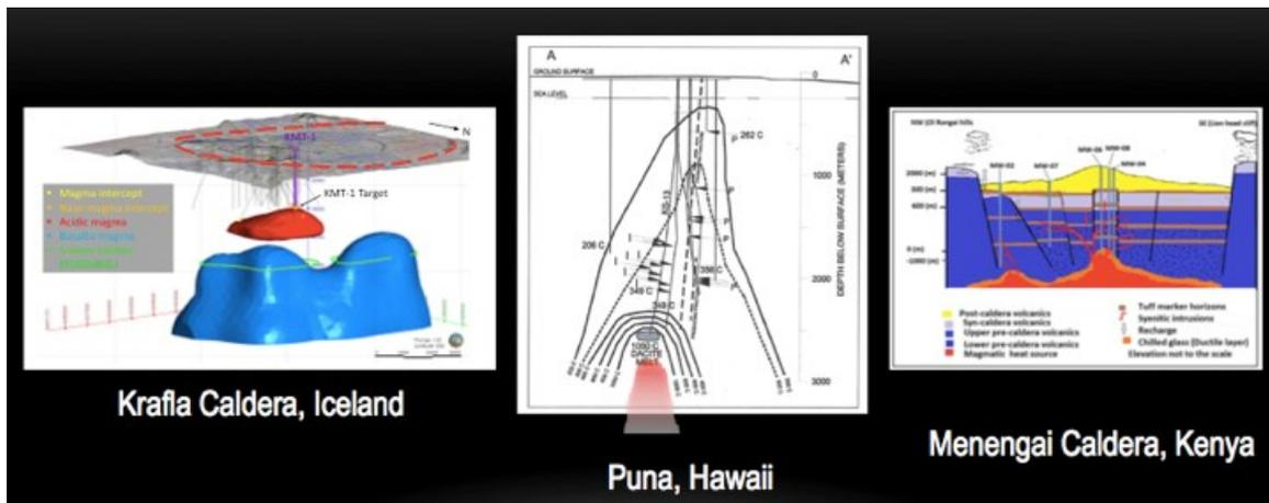
**Figure 1: (L) Plausible model (JW Catley, Reykjavik University) for rhyolitic (red) and basaltic (blue) magma beneath Krafla Caldera (red circle). Geothermal wells (~40) are gray. Planned site and target of KMT-1 are also shown. Two wells penetrated magma and four others may have come close based on temperature and gases. (M) Dacite magma encountered under the lower east rift of Kilauea volcano (Teplow et al, 2009). (R) Syenite magma body centered under Menengai Caldera (Mbia, et al, 2015).**
