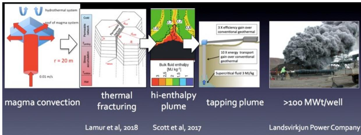
Fig. 8: Idealized scenario for magma-sourced geothermal energy.
