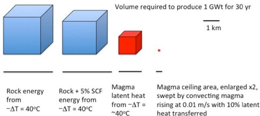
**Figure 4: Comparison of reservoir volumes required to yield  $10^{18}$  J (1 GWt for 30 a). Also shown is area of rising magma column that would deliver 1 GWt for conditions specified (see Fig. 6). SCF is supercritical fluid.**
