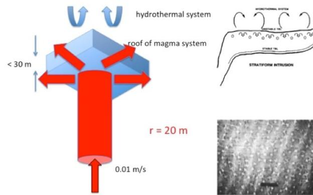
**Figure 6:** Size of “magma heat pipe” required to deliver 1 GWt from 10% of its latent heat to the ceiling of a magma chamber. Relative area needed is shown in Figure 4. Illustrations at right from Carrigan (1984) and Carrigan and Cygan (1986) view and laboratory simulation of multiple convection cells (high Rayleigh number) delivering heat to roof of magma chamber.
