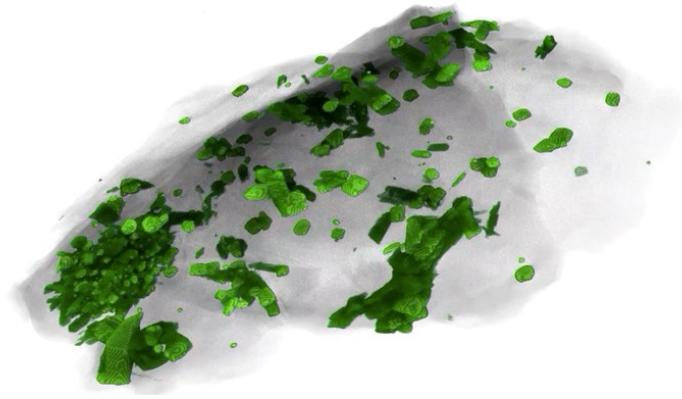
**Figure 2: X-ray tomograph of rhyolite magma quenched at 2100 m depth in IDDP-1 and recovered by circulating drilling fluid. False-color green crystals, mostly plagioclase feldspar, float in transparent melt (now glass) “space”. Long dimension of chip is 3mm. Sample provided by Landsvirkjun (National Power Company of Iceland) and imaged by Fabian Wadsworth at Munich University working with Elodie Saubin, University of Canterbury and Ian Schipper, University Wellington, New Zealand.**
