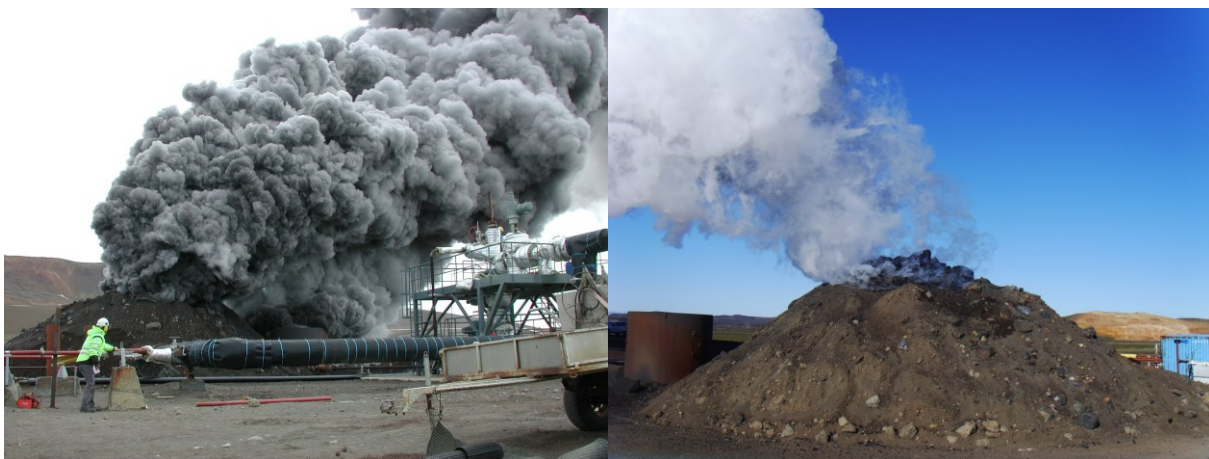
Figure 3: Steam from IDDP 1, beginning of discharge on the left and superheated steam after 30 minutes discharge on the right
