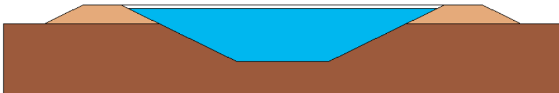
Figure 2: Danish PTES concept with soil balance shaped as a truncated pyramid placed upside down.
