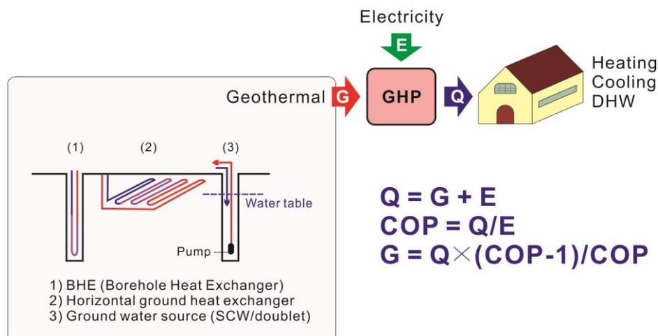
**Figure 1. A conceptual sketch showing how a GHP provides heating, cooling and/or DHW supplies.**
