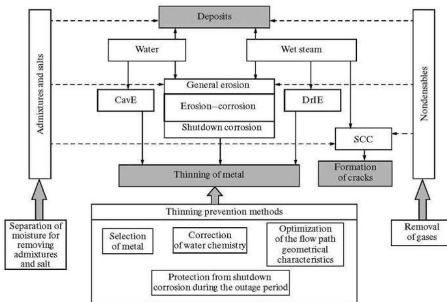
**Figure 1: Problems concerned with damageability of metal and formation of salt deposits in single - and two-phase geothermal heat carriers and methods for preventing damage to elements of GeoPP pipelines and equipment. CavE is cavitation erosion, DrIE is droplet impingement erosion, and SCC is stress corrosion cracking.**
