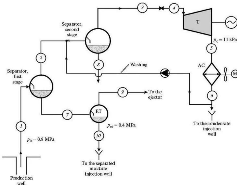
Figure 3: Basic process, circuit of the Merkhne-Mutnovsk GeoPP. (1)—(10) Points at which the concentrations of admixtures in the vapor and liquid phases arc calculated. ET is an expansion tank, AC is an air condenser, M is a motor,  $p_0$  is the pressure at the borehole mouth,  $p_{et}$  is the pressure in the expansion tank, and  $p_c$  is the pressure in the condenser.
