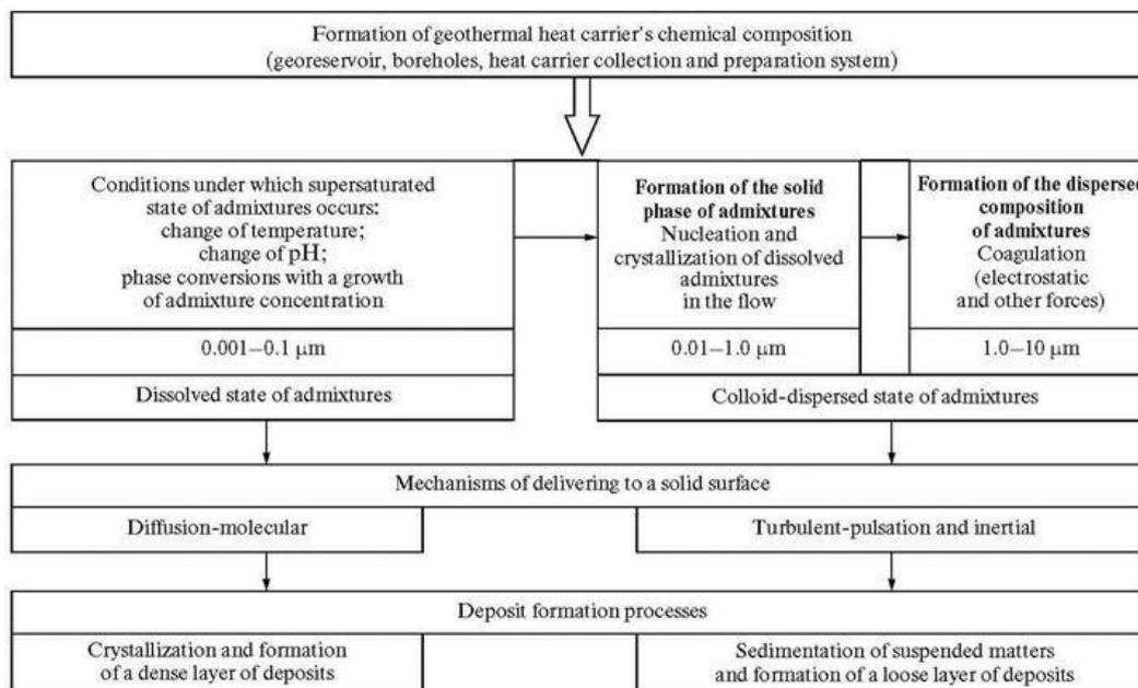
**Figure 2: Conditions, mechanisms, and processes relating to the behavior of admixtures in the GeoPP working loop.**
