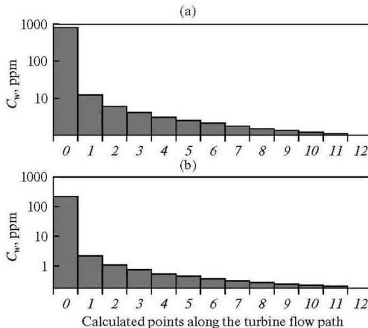
**Figure 5: Calculated concentrations of silicic acid  $C_w$  (a) and chlorides (b) in the liquid phase of working fluid in different flow path stages of the turbine at the Verkhne-Mutnovsk GeoPP.**
