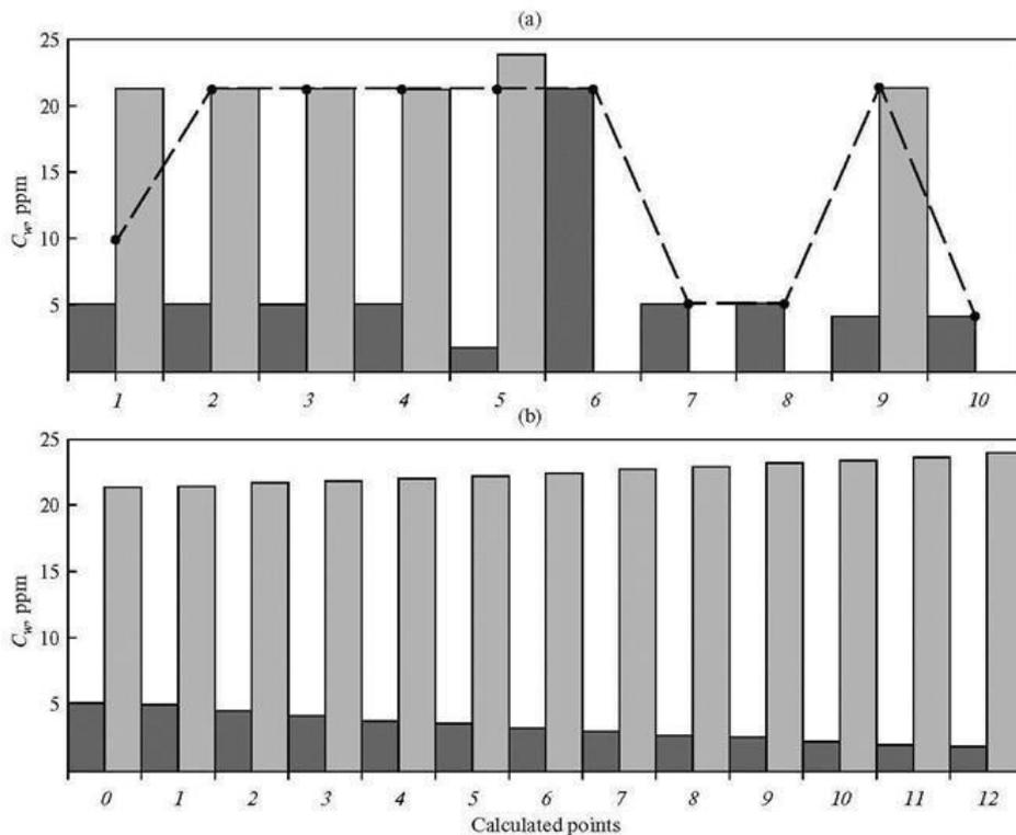
**Figure 6: Calculated concentrations of octadecylamine in the steam and liquid phases of geothermal heat carrier at the Verkhne-Mutnovsk GeoPP (with the octadecylamine concentration at the inlet to the first-stage separator equal to 10 ppm). (a) In the working loop and (b) in the turbine flow path stages. (■, ■) Steam and liquid phases, respectively; and (●) experimental data.**
