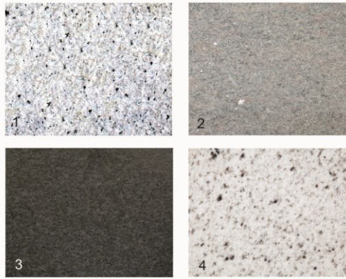
Figure 4: Tested rock samples for ambient spallation drilling. Left-top 1: Gotthard granite, right-top 2: Paradiso migmatit, left-bottom 3: Gabbro granite and right-bottom 4: Bethel granite.
