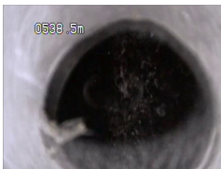
Figure 8: Image taken at a depth of 538.5 m in injection well HN-02 at the CarbFix 1 injection site. The camera enters the injection well through the service pipe (7 in Figure 4). At the time of the photo, CO 2 and H 2 O inlet flows were 27.1 and 750 g/s, respectively. No CO 2 bubbles are visible consistent with the complete dissolution of CO 2 during its injection. (Figure from Sigfússon et al. in review).
