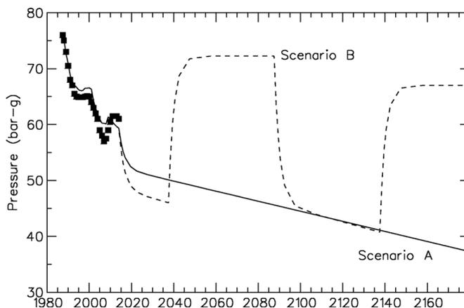
**Figure 2:** An example from Olkaria (Axelsson, 2010) of the ‘cyclic’ development concept. In Scenario B, the short term production is greater (350 kg/s), but cycles on/off. Average pressures are better supported in B than in A, by improving the balance between mass/energy extraction and recharge.
