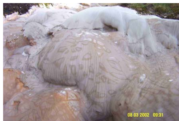
Figure 9. Silica scale deposited in hot-water drains at Wairakei; an example of bacteria-mediated growth patterns.
