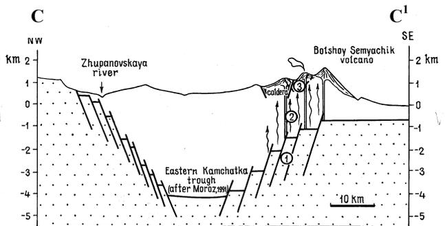
Figure 5. Section showing the location of the volcanoes, thermal manifestations (high-temperature hydrothermal systems) and the position of the basement trough on the Eastern Kamchatka. Legend same as Figure 3.
