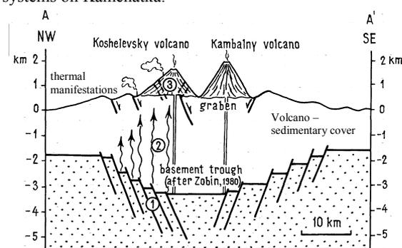
Figure 3. Section showing the location of the volcanoes, thermal manifestations (high-temperature hydrothermal systems) and the position of the basement trough on the extreme Southern Kamchatka. Dotted field is basement (Pre - Cenozoic complex), number in the circles mark the zones: 1 - trough boundary faults - deep structural traps for the magma and hydrothermal fluids, 2 - ascent magma and hydrothermal fluids, 3 - late-Pleistocene - Holocene fissures and normal faults near the surface.
