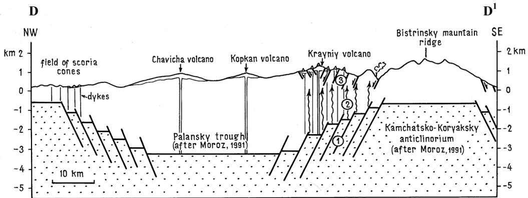
Figure 6. Section showing the location of the volcanoes, thermal manifestations (high-temperature hydrothermal systems) and the position of the basement trough in the centre of Middle (Central) Kamchatka volcanic belt. Legend same as Figure 3.
