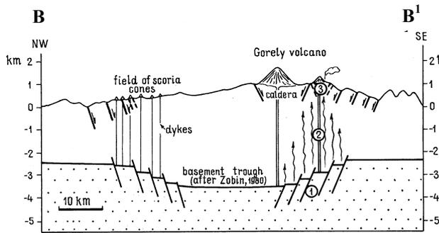
Figure 4. Section showing the location of the volcanoes, thermal manifestations (high-temperature hydrothermal systems) and the position of the basement trough on the north of Southern Kamchatka. Legend same as Figure 3.
