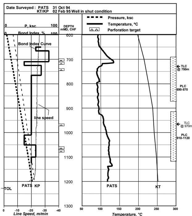
Figure 1. CBL, electronic temperature and pressure and KT/KP profiles used to refine perforation targets.
