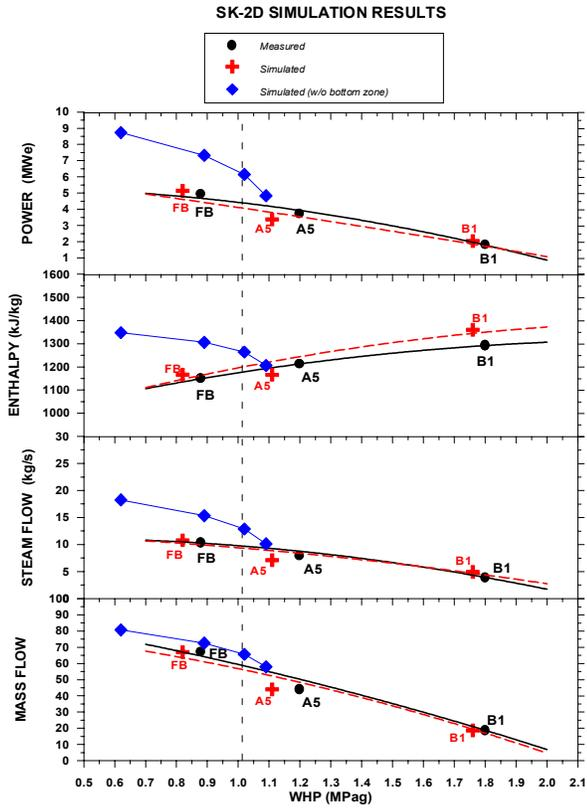
Figure 3. Bore output measurements for SK-2D at different wellhead conditions.
