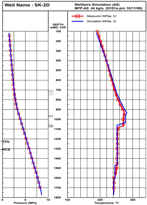
Figure 5. Results of wellbore simulation while discharging at 1.20 MPag wellhead pressure.
