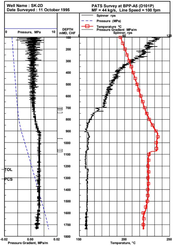
Figure 4. PATs log of SK-2D while discharging at 1.20 MPag wellhead pressure (BPP A5).
