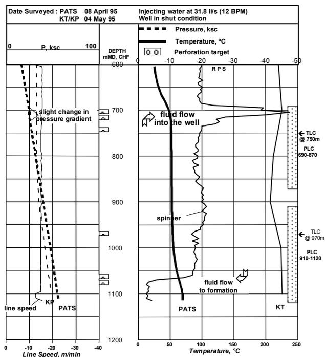
Figure 2. Results of post-perforation completion test with bridge plug set near the production casing shoe.
