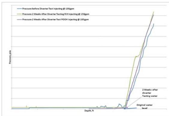
Figure 10. Pressure vs. Depth Comparison two-weeks after diversion
