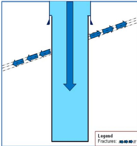
and then temporarily isolate those fractures hydraulically while a second set of fractures is stimulated. One could attempt to do this with some type of mechanical isolation tool such as an open hole packer (See **Figure 2**), but this would require that a drilling rig be present during the stimulation treatments. This would incur additional costs as well as the associated operational risk of packer failure (i.e. getting the packer stuck in the hole, etc.)
