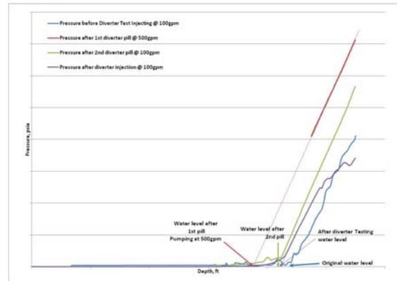
Figure 8. Pressure vs. Depth
