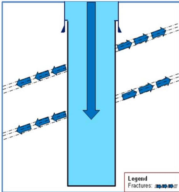
This same method of using chemical diverters could be used in the stimulation of conventional hydrothermal wells as well: The existing producing fractures would first be stimulated (if desired), then a temporary diverter would be pumped in to seal off the existing fractures. Afterwards, additional hydraulic pressure would be applied, and additional fractures would be stimulated to improve production from the well.
