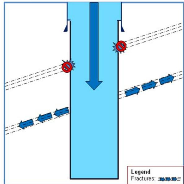
Figure 4: EGS Well with Multiple Fracture Networks
