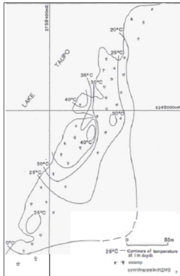
Figure 3. Map of temperature contours at 1 m depth (Bibby et al. 1991, after Fisher, 1957)
