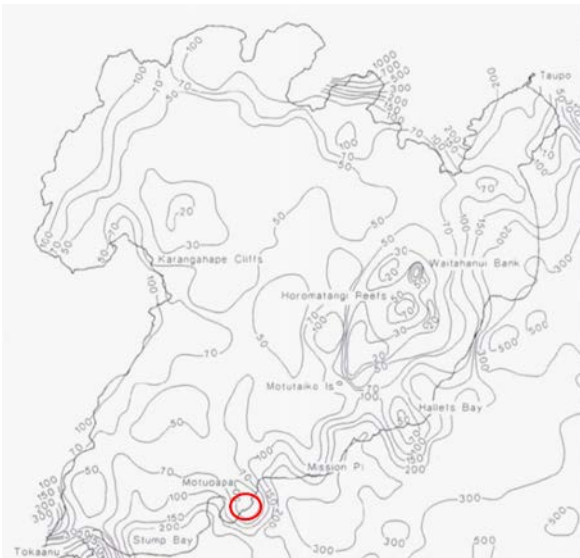
Figure 4. Apparent resistivity contour map of L. Taupo with Motuapa circled in red (from Bibby et al. , 1991).
