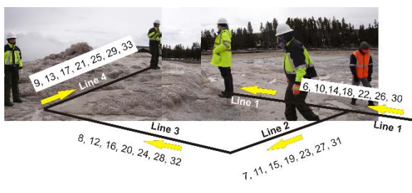
Figure 2: Four time sequence transect lines (Lines 1 to 4) located on western slope of Old Faithful geyser. Seven GPR runs were performed along the four lines at different time intervals (see Table 2). Numbers represent each GPR run.
