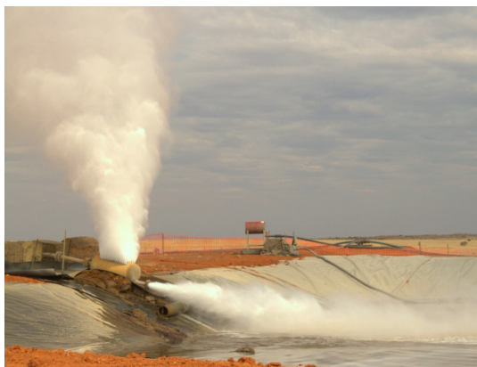
Figure 4: Open Flow Testing of Habanero 4 (source GDY Internal)
