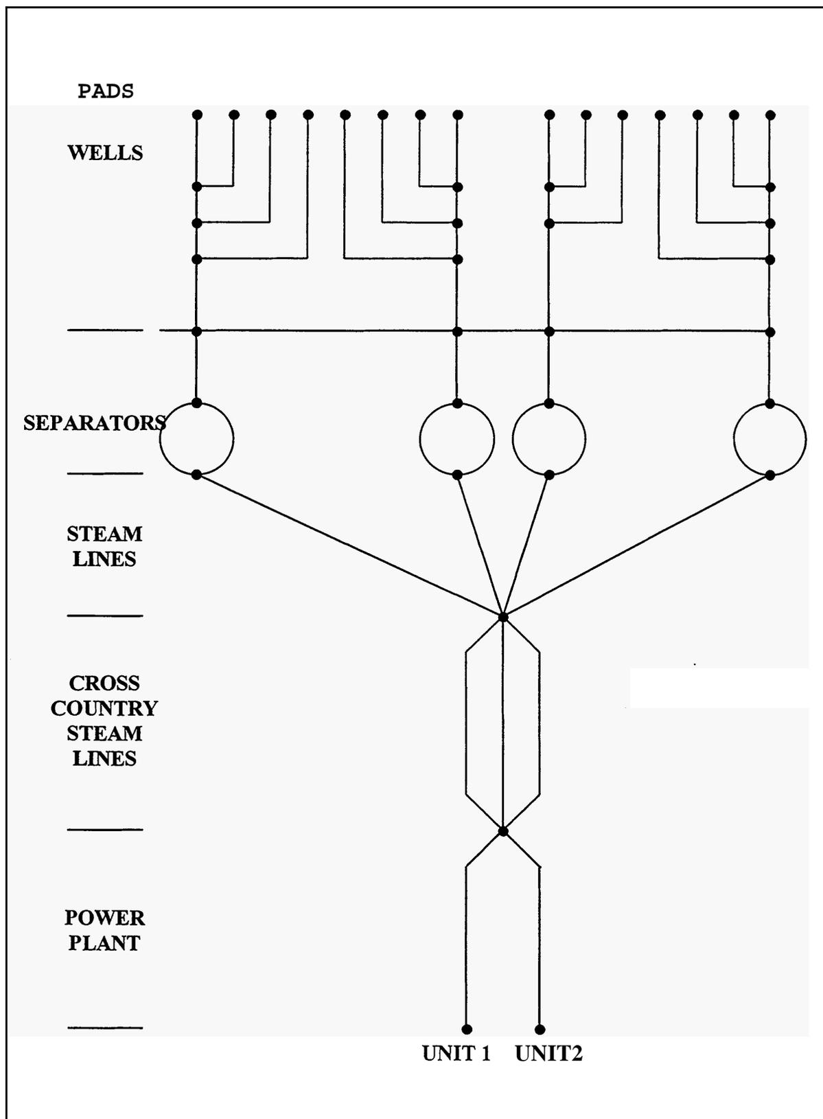
Figure 1 Steamfield Schematic
