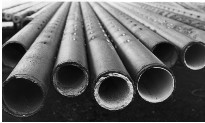
Figure 9. Calcite scaling in Krafla well liners
