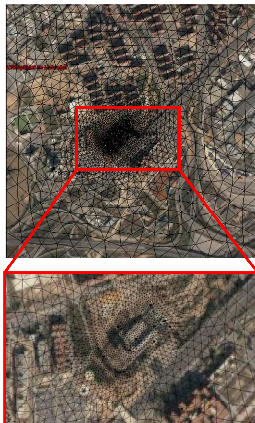
Figure 5: Discretisation of the area. The figure shows a plan view of the finite element mesh within the domain (up) and a detail of the mesh refinement in the vicinity of the hotel (down).
