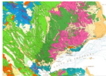
Figure 2: Extracted from the geological map of central and southern Afar (J.Varet, 1975). The Mabla rhyolites (violet), are faulted along the Red Sea direction and covered after erosion by the basaltic Dalha plateau (deep green), itself intensively faulted and tilted towards NW, eroded and covered by the Afar stratoid series (clear green). In the vicinity of the Gulf of Tadjoura, these faulted and eroded blocks are covered by the basalts emitted during the early stage of opening of the Tadjour oceanic ridge (blue-green), deeply faulted along Aden rift normal and transverse directions. Bathymetric contours in the gulf are also drawn showing the position of the ridge near the Obock coast.
