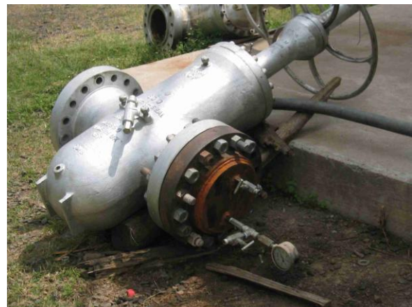
Figure 7 Hydrostatic pressure testing of reconditioned valve
