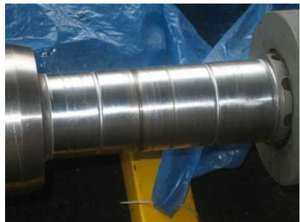
Figure 5 Worn turbine rotor shaft
