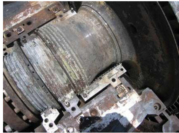
Figure 3 Worn rotor labyrinth steam seal
