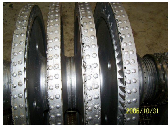
Figure 4 Corroded shroud bands
