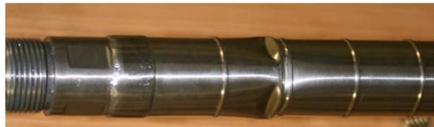
FIGURE 4: On the figure a dent on the capillary tube can be seen. This part of the tool is shielded from heat, pressure and geothermal fluid when logging is ongoing. The damage occurred due to too high speed. Though the tool did not stop abruptly on an obstruction in this case, speeds above ~35m/min. are enough, in deviated well, to do this kind of damage.
