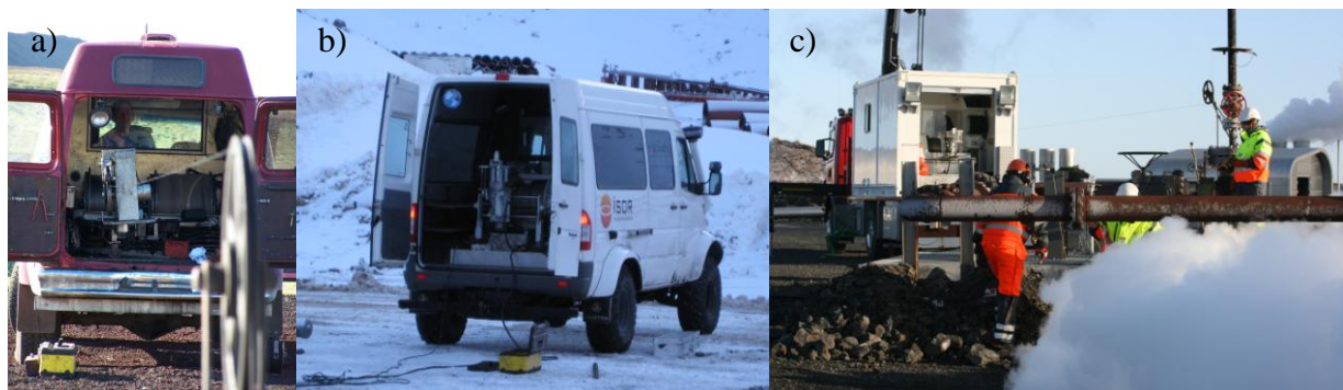
Figure 6: The “fleet” of three slick-line logging trucks, in action, that Iceland GeoSurvey currently operate. a) The 1997 Ford Econoline, double winch slick-line and e-line truck, b) the 2006 Mantra slick-line truck and c) the 2008 Scania double winch slick-line truck.
