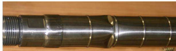
FIGURE 4: On the figure a dent on the capillary tube can be seen. This part of the tool is shielded from heat, pressure and geothermal fluid when logging is ongoing. The damage occurred due to too high speed. Though the tool did not stop abruptly on an obstruction in this case, speeds above ~35m/min. are enough, in deviated well, to do this kind of damage.
