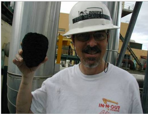
In this photograph taken at Bouillante II in the West Indies, Tom McAuliffe holds a lump of mineral scale removed from plant equipment. The potential for scaling is one of the design challenges that set geothermal plants apart from more conventional plants.
