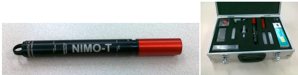
Figure 12: Pressure and temperature logger NIMO-T, and setup for precise temperature logging.
