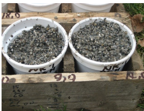
Figure 3: Rock mass samples collected during drilling at 9.0 and 10.0 m.
