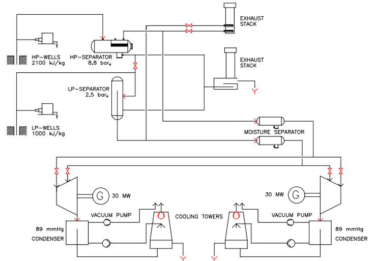
**Figure 4.** The principles of the process for the present 60 MW power plant
