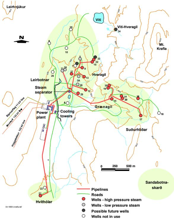
**Figure 3.** Schematic map of the Krafla geothermal power plant and the surrounding area.
