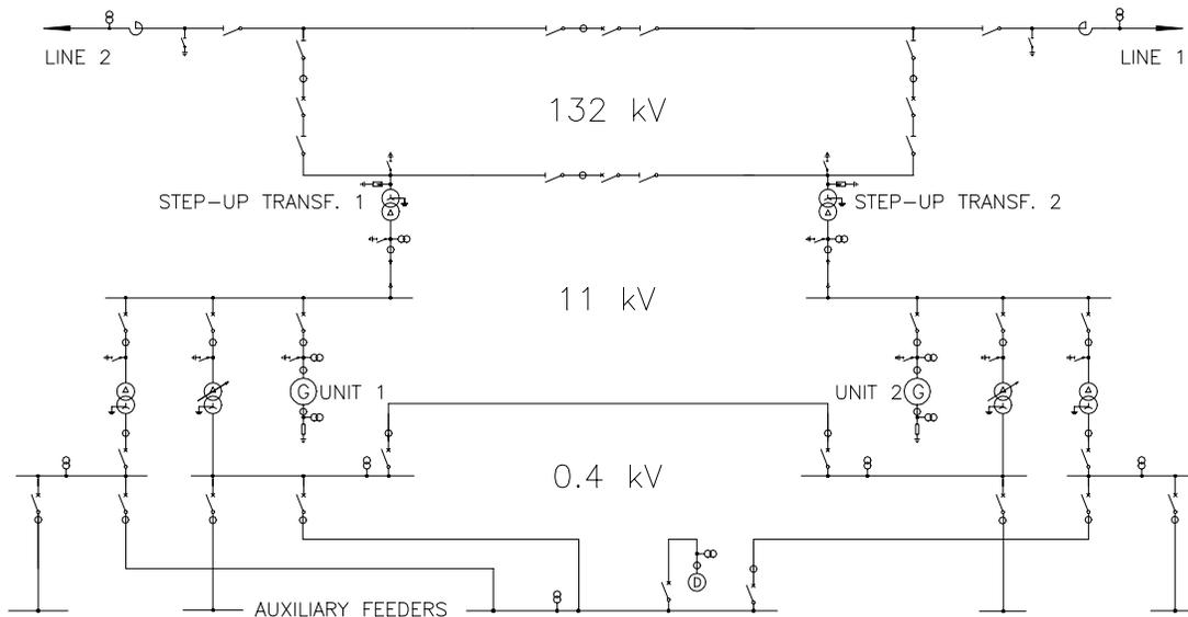
**Figure 5.** Design concept of the main electrical power system after the erection of unit 2.
