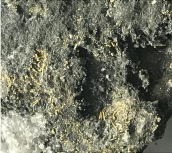
**Figure 2: Vatoukola high-grade gold ore where quartz minerals and gold needles can be seen in the porous basalt.**
