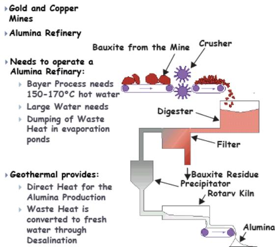
**Figure 1: Geothermal energy provides multiple opportunities for mineral recovery and processing. The alumina refinery is an ideal example of where the same geothermal heat can be used twice.**
