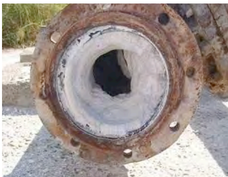
Figure 4. CaCO 3 scaling formed in KD 13.
